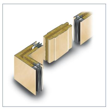
Detail for changing direction of installation
