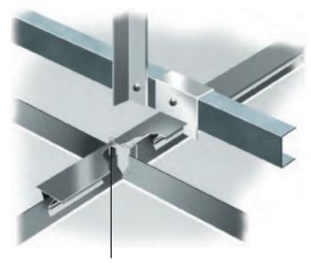
Security clip GT1071 hooks into the four adjoining tiles at corner locations and secures tiles to grid over the tee bars GTII5
