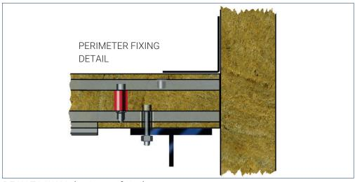
DECK TO WALL (perimeter fixing)
