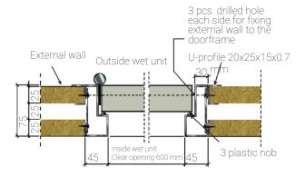
As standard the external linings slide into the door frames.
