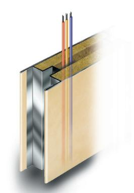
Air gap for installation of cables.
