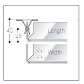
TYPE 'A' TILE 5mm Bevel edges to all sides.
