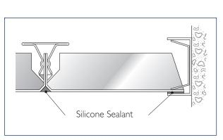
SECTION SHOWING AIR AND DUST TIGHT CEILING
