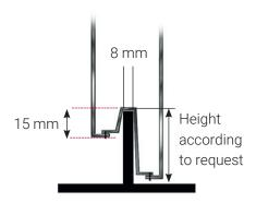
Standard thickness of flat bar 8 mm, others are available. Flatbar is normally part of the yard's delivery.
