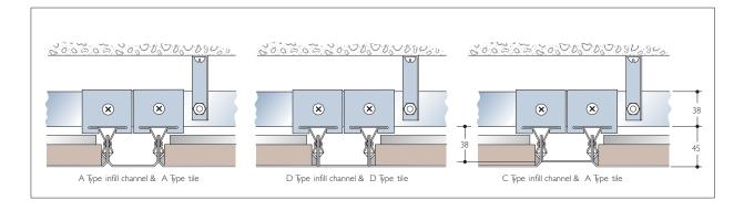
We only recommend the use of Burgess Tee Bar for this system. Each piece of Burgess Tee Bar is identified as such on the rear face.
