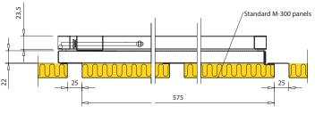
SECTION A-A, INSULATED FOR B-0 RATING.
