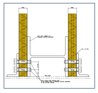
Typical periphery fixing detail
