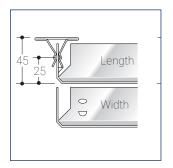
TYPE 'A' TILE 5mm Bevel edges to all sides.
