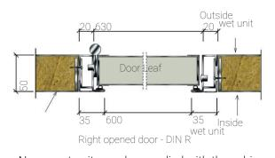
Norac wet units can be supplied with the cabin side having a finished surface as shown above.
